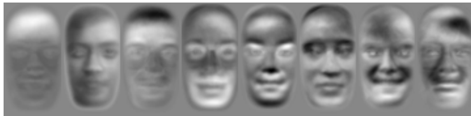
Figure 3.1. “Eigen-faces” – eigenvectors corresponding to the eight largest eigenvalues of a set of face images. The brightness of each pixel represents the magnitude of a coefficient. Zero-valued coefficients are rendered in intermediate gray; large positive and negative coefficients in white and black, respectively. (Reproduced with permission from Moghaddam and Pentland [72].)
