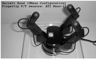
Figure 2: The Barrett Hand has four DOFs. These include one flexion DOF for each of the three fingers and one adduction DOF. The adduction DOF spreads two of the fingers about axes in the palm.
