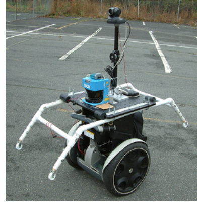
Fig. 3. The Segway RMP equipped with a laser range finder and a camera. The PVC pipes are a safety system that protects the on board equipment from damage in case of system failure.
