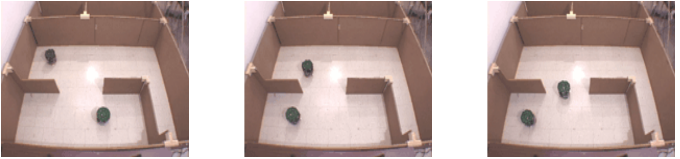
Figure 2: A two robot leader/follower coordination primitive in action. The lower robot is the leader and is moving right to left.
