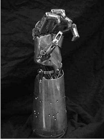
Figure 1. Robonaut hand without glove
