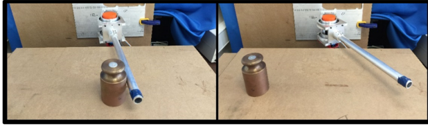
Fig. 16 The SEA prototype with a low impedance setting causes the link to be obstructed (left). Increasing the control impedance overcomes the obstruction (right), shown after the object has been moved and the arm retracted.
