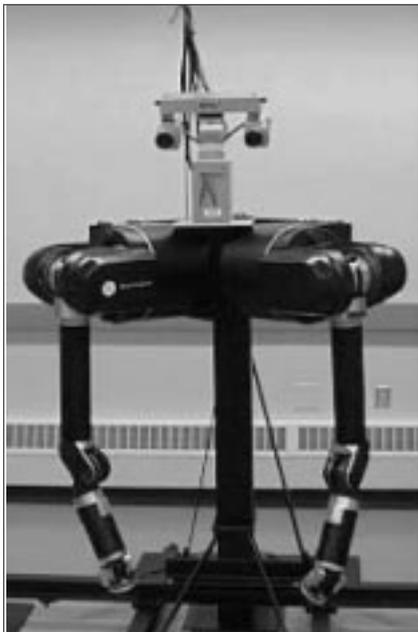
Figure 1. Magilla's current configuration. Barrett Technologies designed and built the arms and hands.
